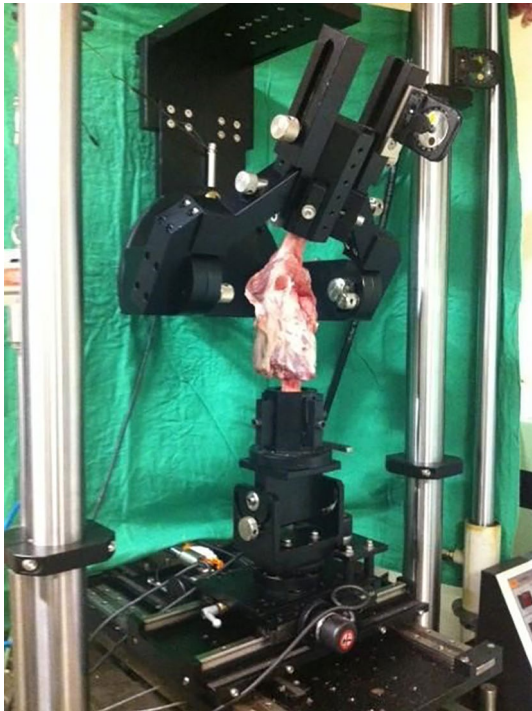
Fig. 1 Porcine knee specimens mounted on the Instron testing machine (Instron 8501, MTS, Minneapolis, Minnesota)
